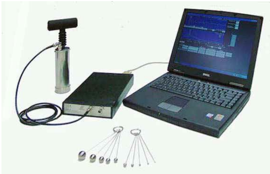
Figur 7. Typisk slag-eko provutrustning, impact echo test system, Impact-Echo (2016)
